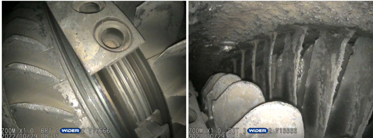
Figure 3: Damaged HPC 6th Stage
