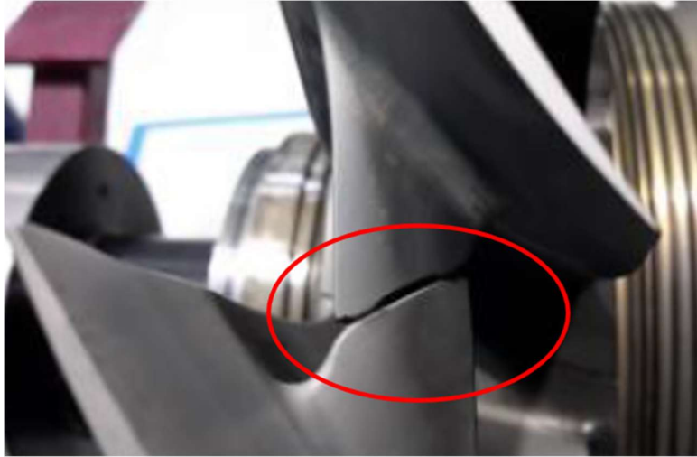
Figure 11: Extensive clapper wear
