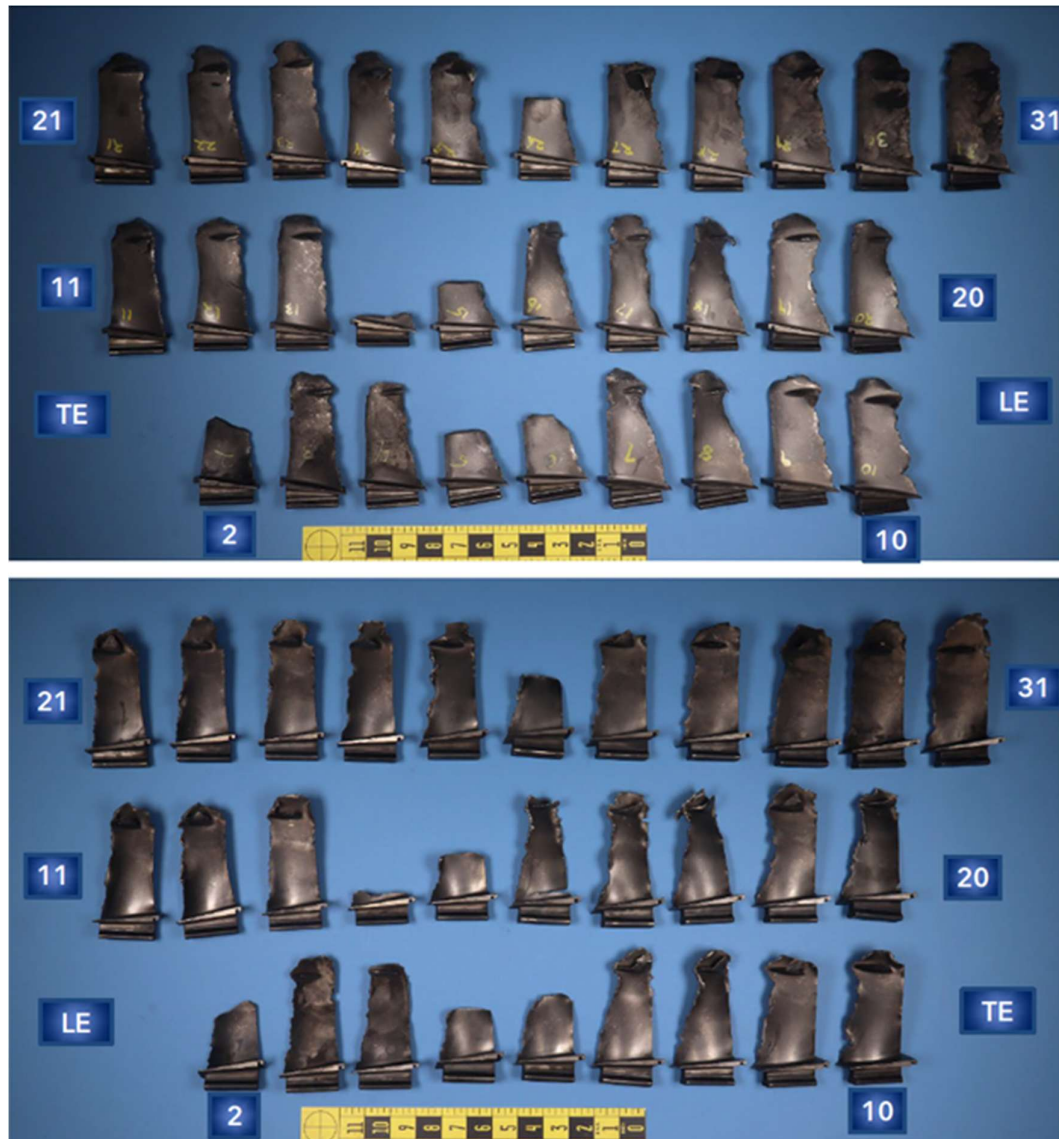
Figure 22: concave side (upper image) and convex side (lower image) of the HPC 3rd stage blades 2-31 positioned consecutively. LE- Leading edges and TE- trailing edges.
