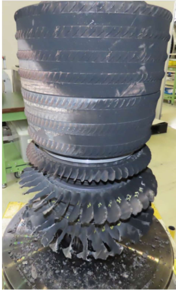
Figure 17: Damaged HPC all Stages
