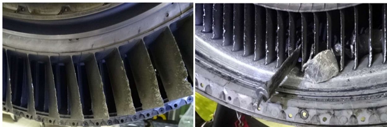
Figure 16: Damages in LPC 2.5 Blade (LH) and in LPC 2.5 vanes (RH)
