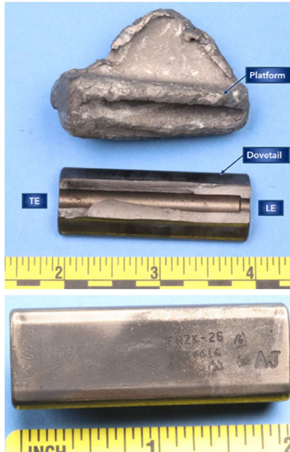
Figure 21: Blade no. 1 showing the dovetail piece and mating piece with the platform and airfoil root (upper image) and the root end face of the dovetail (lower image).
